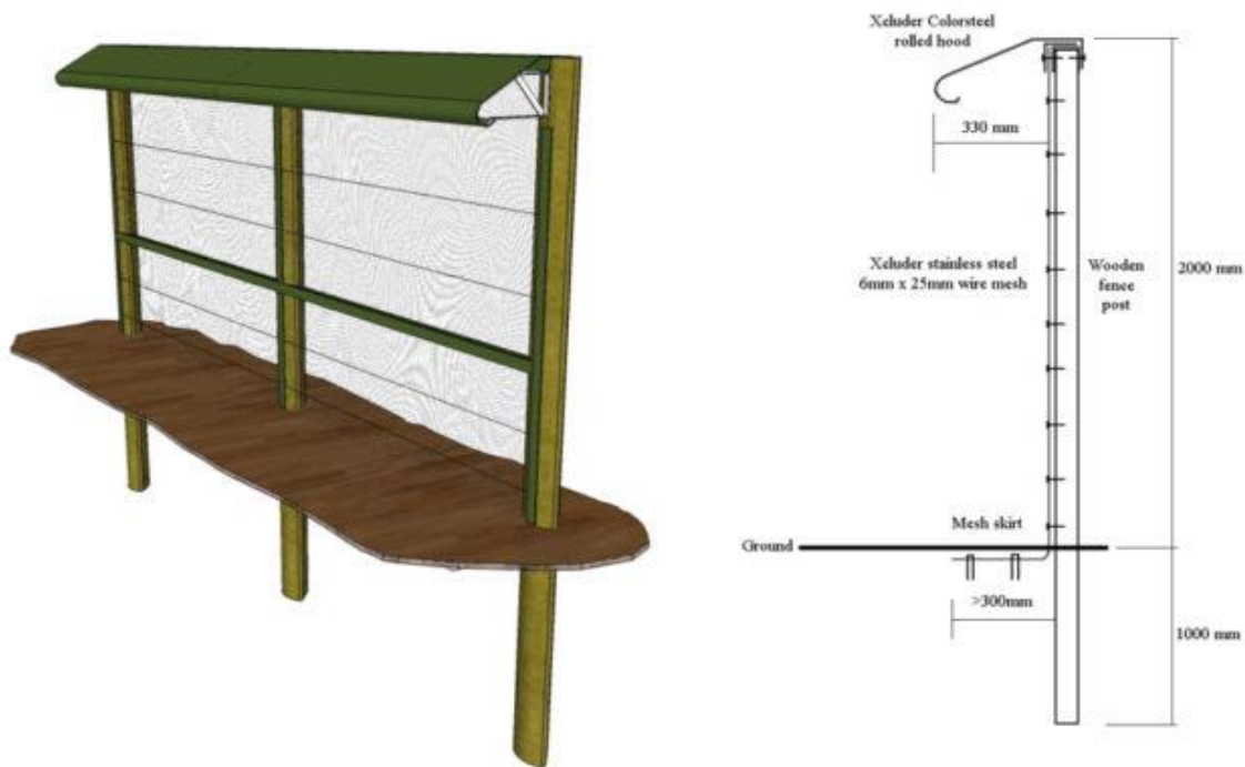
Image 73. General pest and predator-proof fence design. © Dep. of Conservation, NZ, Bell 2014.
